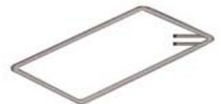
**Figure 2:** Steel reinforcement in seismic columns ties with 135 degree hooks
